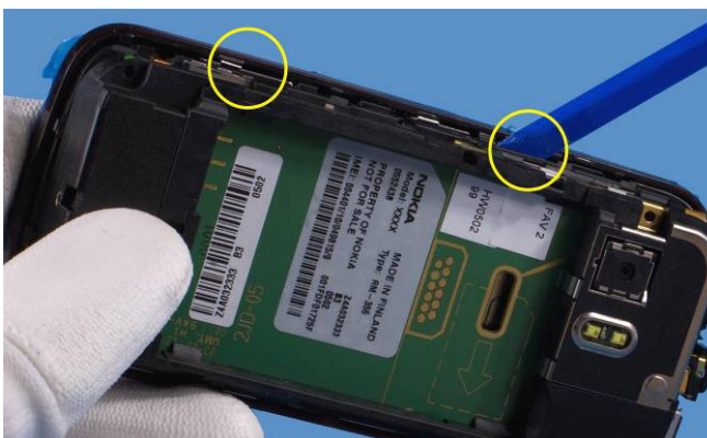
11. Go on releasing the snaps on both sides of the phone.
