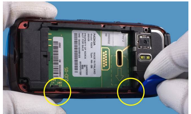
4. Release the snaps of the SIDE BAND ASSY with SRT-6 .
