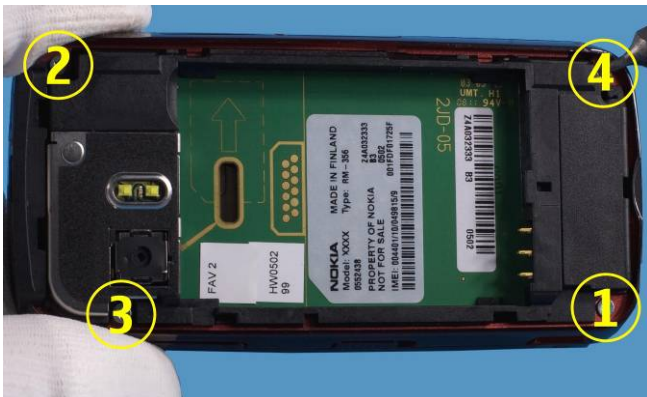
3. Unscrew the four TORX5+ screws.
