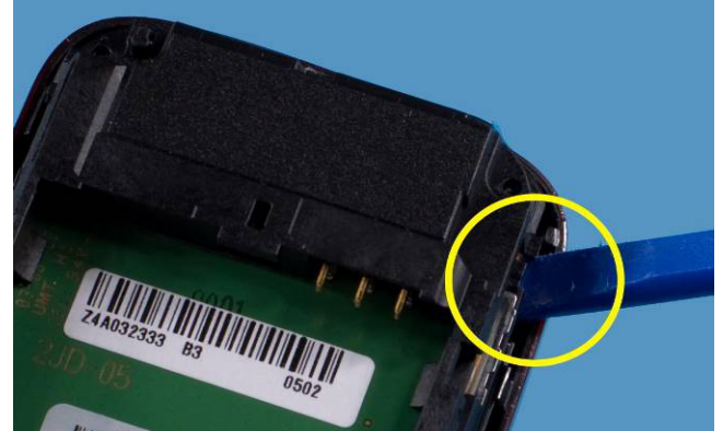
8. Release the snap of the A-COVER in the bottom corner as shown in the picture with SS-93 tool.
