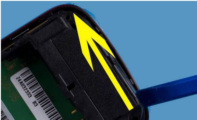
9. Slide with SS-93 tool along the bottom side to release the snaps here as well.
