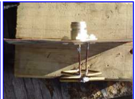
Looking down on it when it is aligned for horizontal polarization (i.e. the diamonds are vertical)
